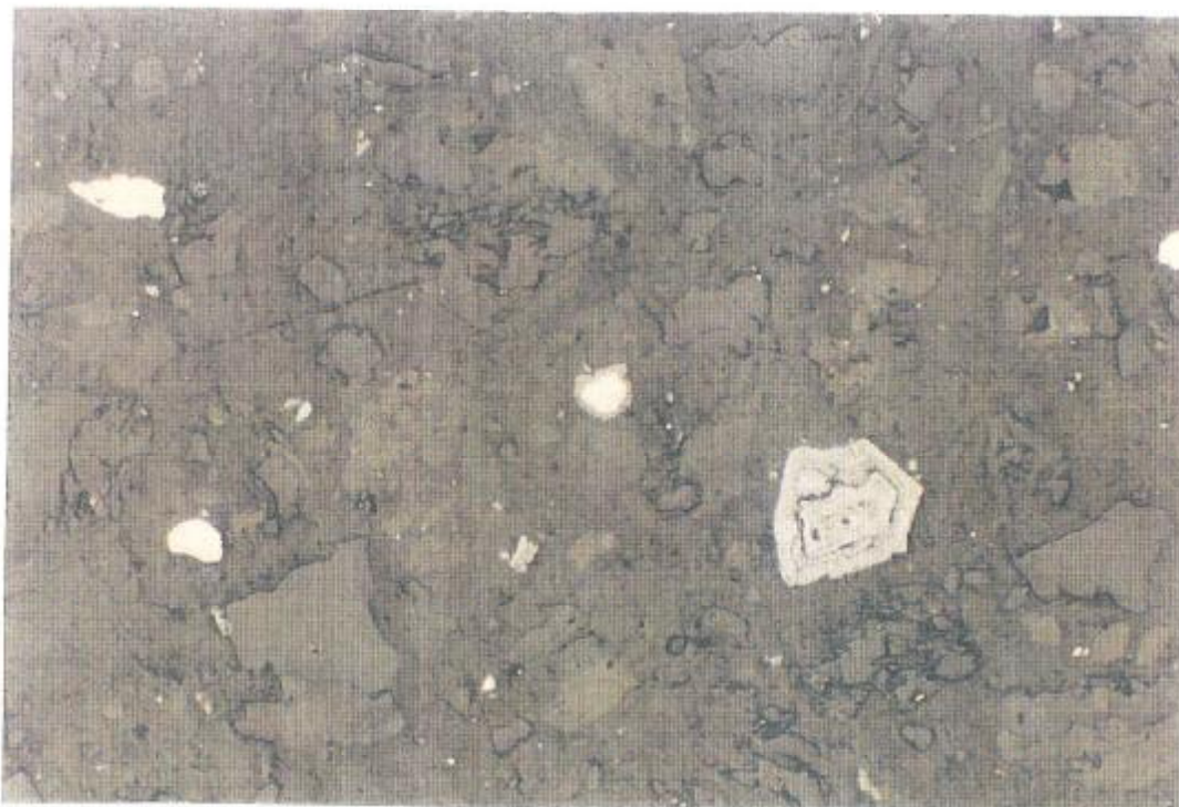
Figure 19. Sample TCP-01 in plain reflected light, width of field 0.625 mm, showing a zoned grain of roaster-type Fe oxide. To its left is a grain of pyrite that is rimmed by Fe oxide, indicating that roasting did not consume some of the sulfide grains. Whitish grains to the left and far right are unoxidized pyrite, presumably from the flotation tailings.
