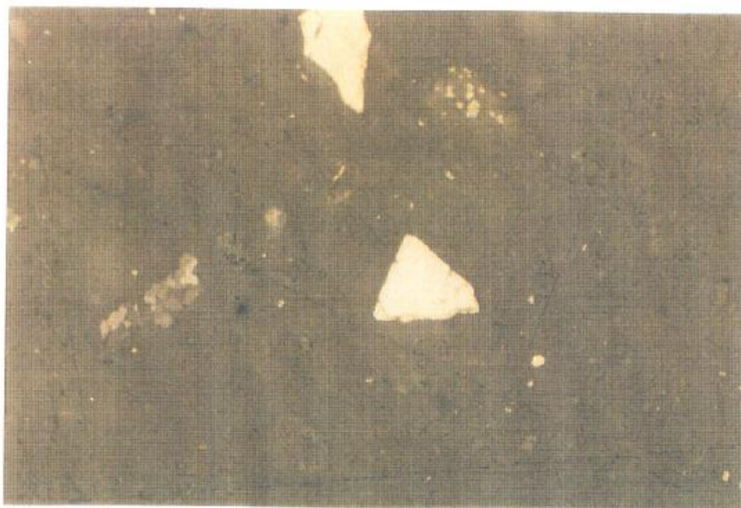
Figure 27. Sample TNW-01-05 in plain reflected light. Upper photo (width of field 0.625 mm) shows one of the few particles of zoned Fe oxide (right of centre) in the sample. The large, whitish sulfide grain on the left is pyrrhotite. Lower photo, width of field 0.3 mm, shows a triangular grain of pyrite, apparently with a narrow, barely visible reaction rim.
