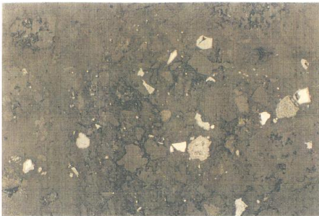
Figure 22. Sample TNP01 in plain reflected light, width of field 0.625 mm, showing roaster-type oxides, some with unconsumed sulfide cores.
