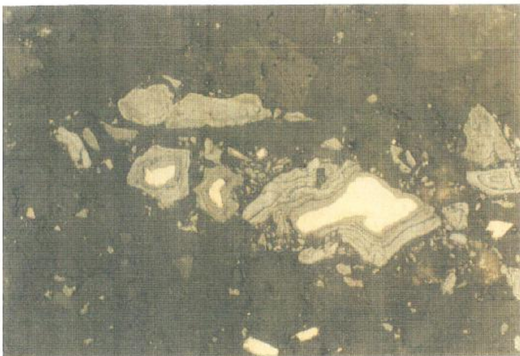
Figure 20. Sample TCP-01 in plain reflected light, width of field 0.3 mm, showing roaster-type oxides, some with unoxidized cores of pyrite.
