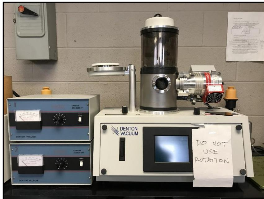
*Figure 2-19 - Carbon coating equipment - vacuum chamber with carbon coating accessory on top (right), and source of current (left).*
