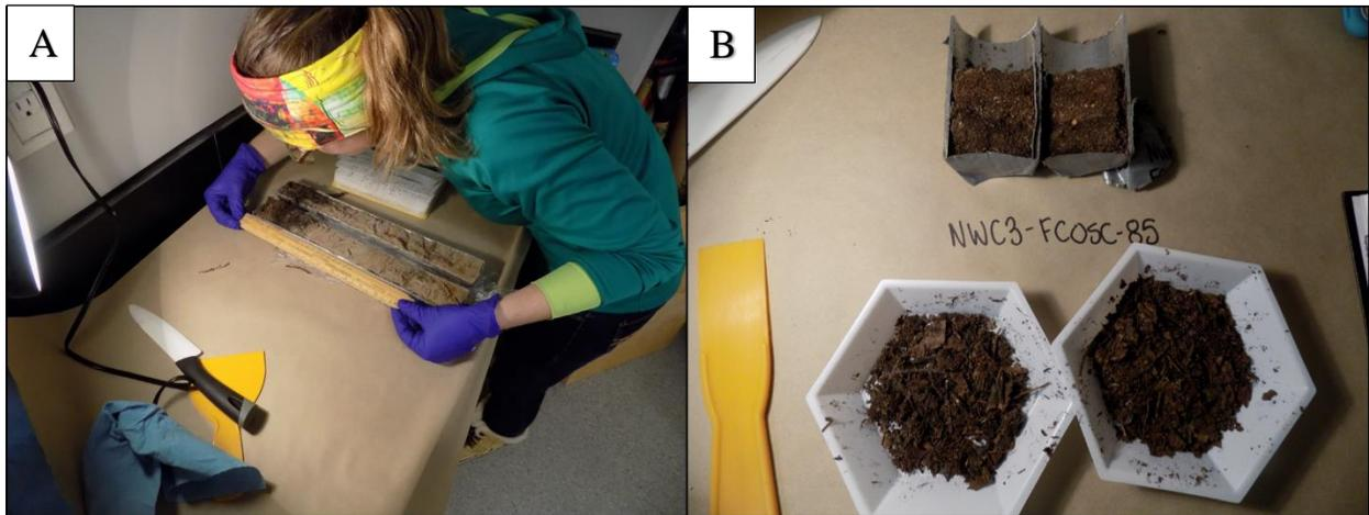
Figure 2-13 - A: Split soil core being measured prior to being sub-sectioned using a ceramic blade (shown in photo). Notes were recorded regarding the changes in soil texture, colour and composition at various depth intervals. B: Sub-sectioned public health layer (0 to 5 cm, taking compression into account) samples were transferred to plastic weight boats and homogenized before being split into Ziploc bags.
