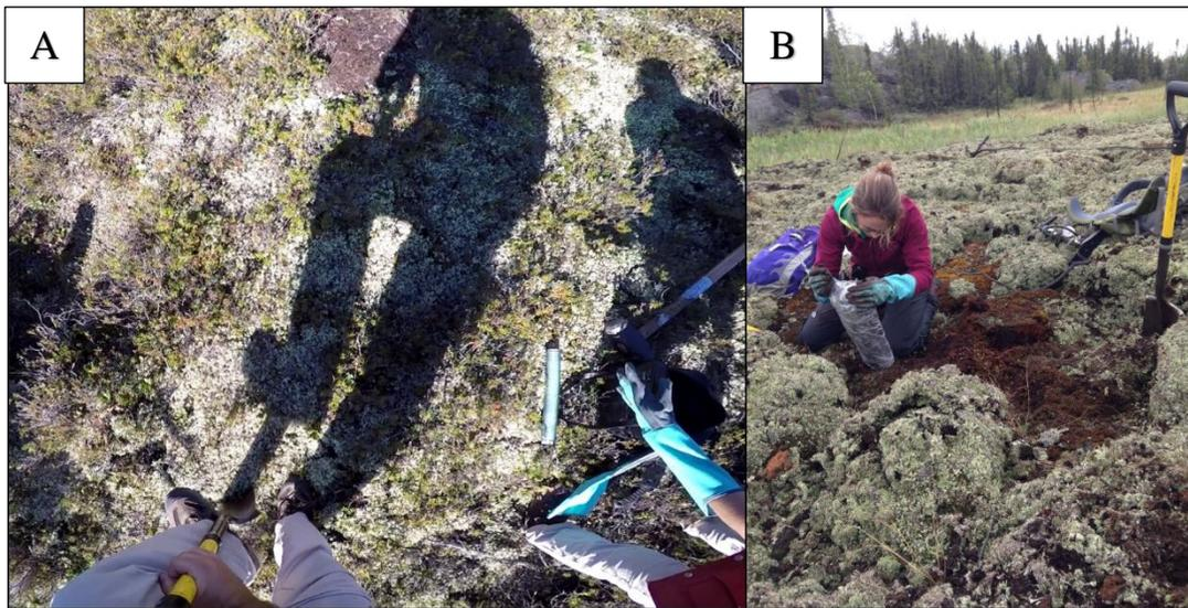
*Figure 2-11 - A: Shovel being used to extract a section of peat. B: After removing the peat core from the ground, it was wrapped in plastic wrap and labelled.*
