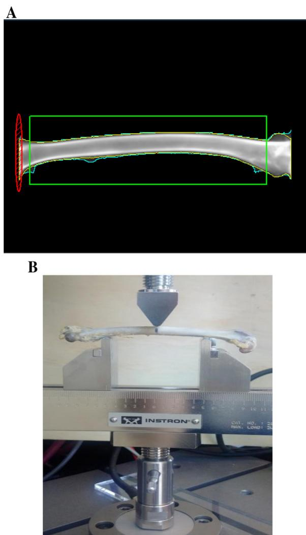
**Fig. 1.** a: Delineation of the region of interest (ROI) for bone densitometry measurement b: Test setup of a femur sample placed on a three-point bending jig, with mid-diaphysis (marked) aligned with the load application point, and 5 cm from bottom supports.
