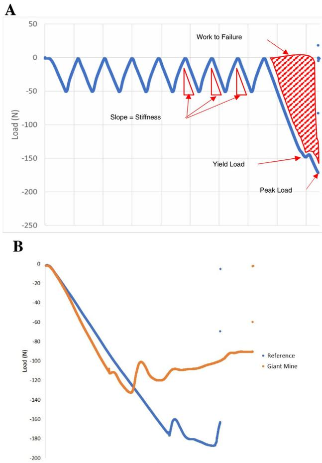
**Fig. 2.** a: A sample load curve, each specimen was cycled from 2 to 50 N in three-point bending (compression being negative load) eight times, followed by a constant displacement ramp load to failure. The slope of the line for the last three cycles was calculated for stiffness, and the yield load, peak load, and work to failure were identified as shown. b: Representative load curves of work to failures of snowshoe hares bones from two locations.
