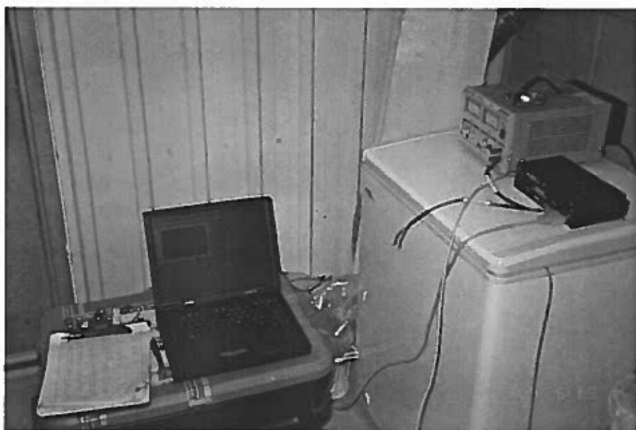
Photograph 2: TDR test set-up: TDR100 unit and power supply (upper right corner and sitting on chest freezer) connected to laptop and TDR probe.
