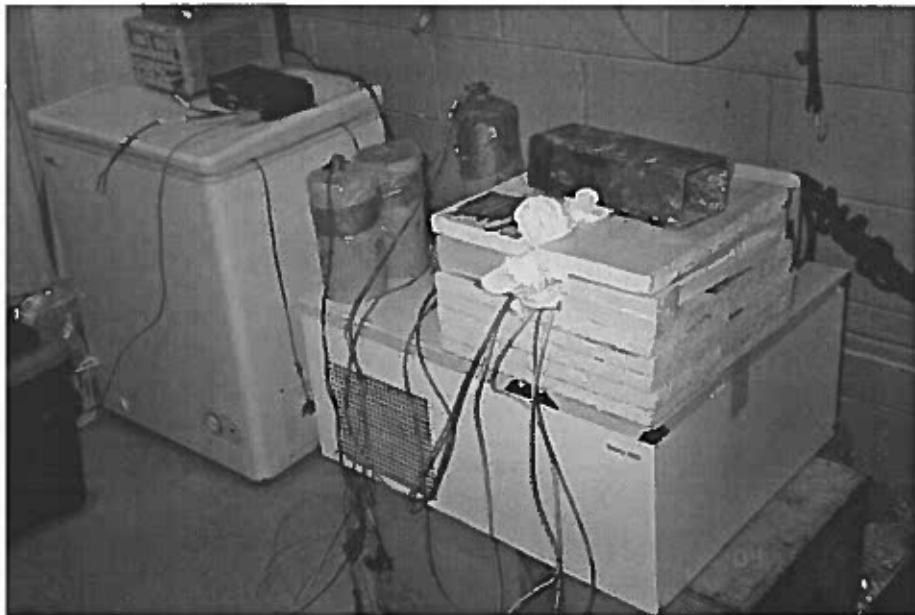
Photograph 3: TDR test set-up: Isotemp 3028 circulation bath with specimens stored in work area beneath the Styrofoam insulation and probe leads extending to the TDR100 unit (background).
