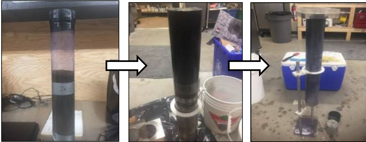
Figure 2.2 Sediment core slicing process into 1-cm sub-sections via a gravity corer ( Unwitec ).
