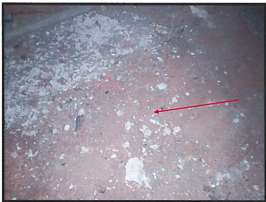
Photograph 6: Non-Asbestos Insulation Debris on Basement Level, Suspected to be From the Ceiling (Sample 40).
