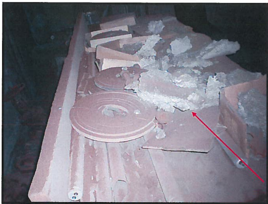
Photograph 9: Spray Applied Ceiling Insulation Debris on Table (Sample 09).
