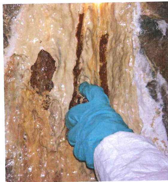
Figure 5. (for color see Plate 11) Biofilm developed on underground stope wall where As-rich water drips from an drillhole. Mineral precipitate is yukonite \text{Ca}_7\text{Fe}_{12}(\text{AsO}_4)_{10}(\text{OH})_{20} \cdot 15\text{H}_2\text{O} .
