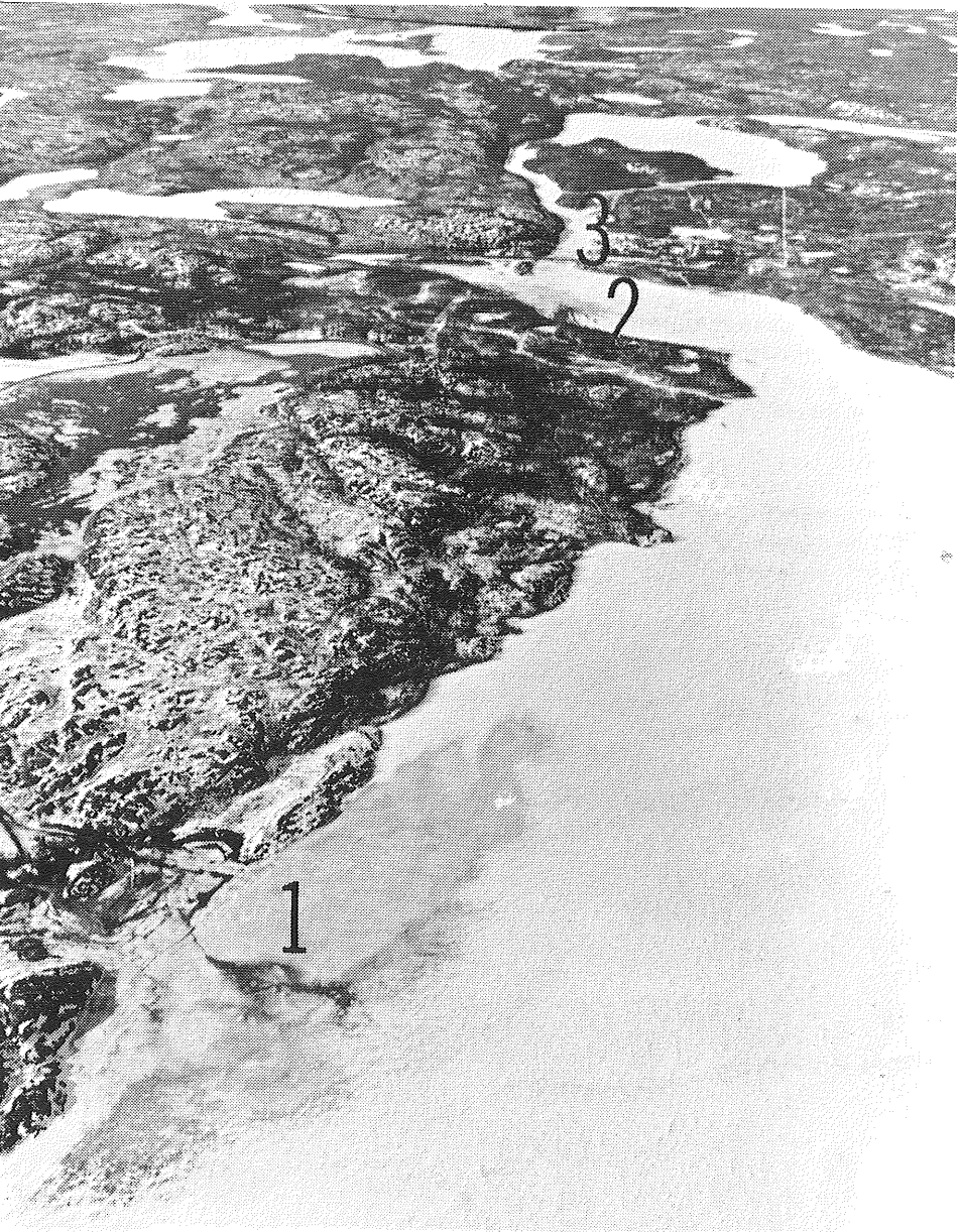
This photo shows Giant Mine's tailing seepages in April 1974 and their relation to the Yellowknife water supply. Point #1 shows the spill while #2 indicates the area where seepage has continued for a number of years. Point #3 pinpoints the position of Yellowknife's present water intake system installed in 1970 and located in the Yellowknife river. The old water intake [lower right of photo] is located in the middle of Yellowknife Bay and in the event of an emergency, water from this polluted area would be fed directly into our existing system.
