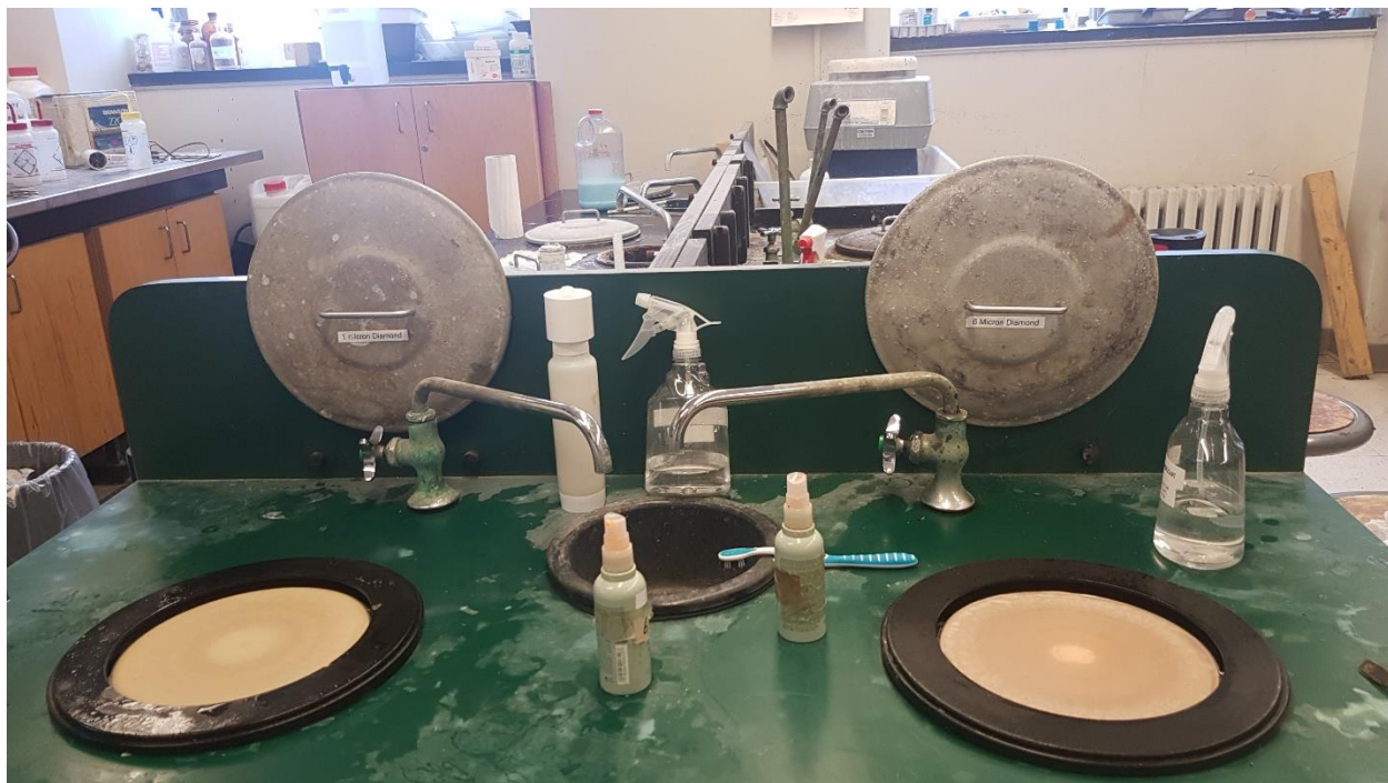
Figure H-4: Final two steps of polishing; on the right, 6-micron diamond polish is done first and then, on the left, 1-micron diamond polish.
