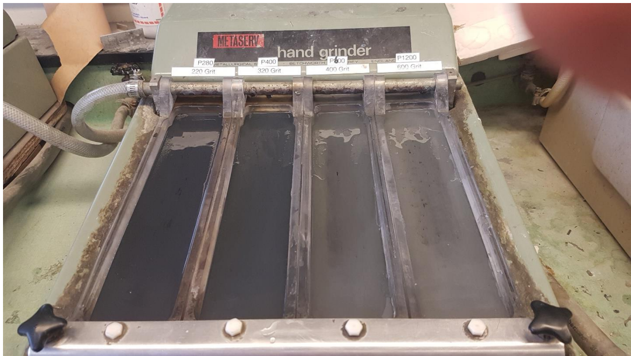
Figure H-3: Polishing on grit 220, 320, 400, and 600 sandpapers.
