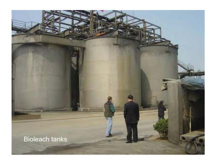
REBgold's bioleaching technology employs the use of naturally-occurring bacteria, harmless to both humans and the environment, to liberate precious and base metals from difficult to treat ores, concentrates and tailings produced by the mining industry. REBgold is one of only two companies to have successfully commercialized gold bioleach technology. By virtue of having no direct competition, the company is the leader in the base metal bioleach arena as well.
