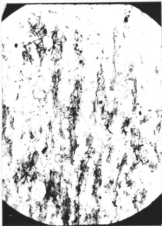
Fig. 11 - Chlorite lenticles with rutile needles. X 70
