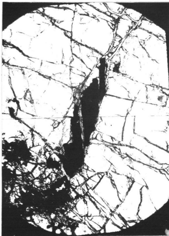
Fig. 24 - Sulphides in garnet X 70
