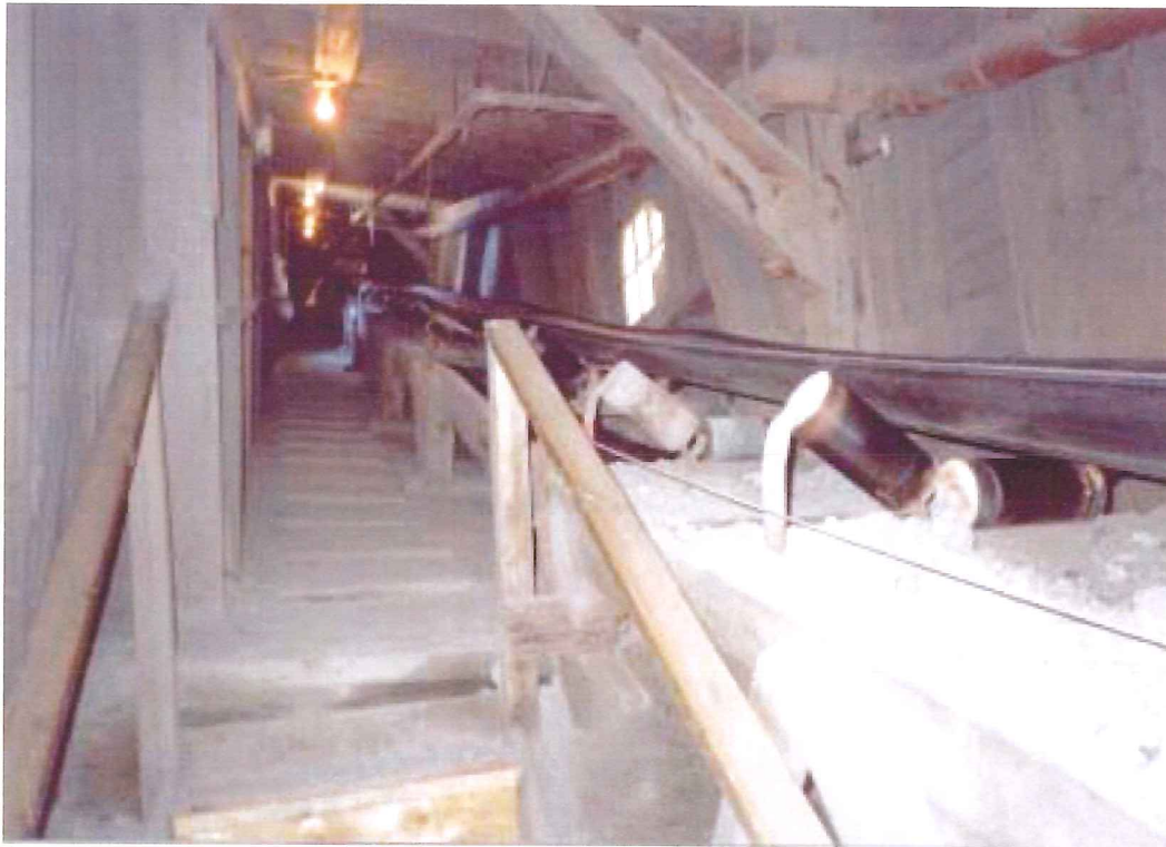
Interior Towards Screen House from Crusher House (Note: Conveyors are made of Wood)
