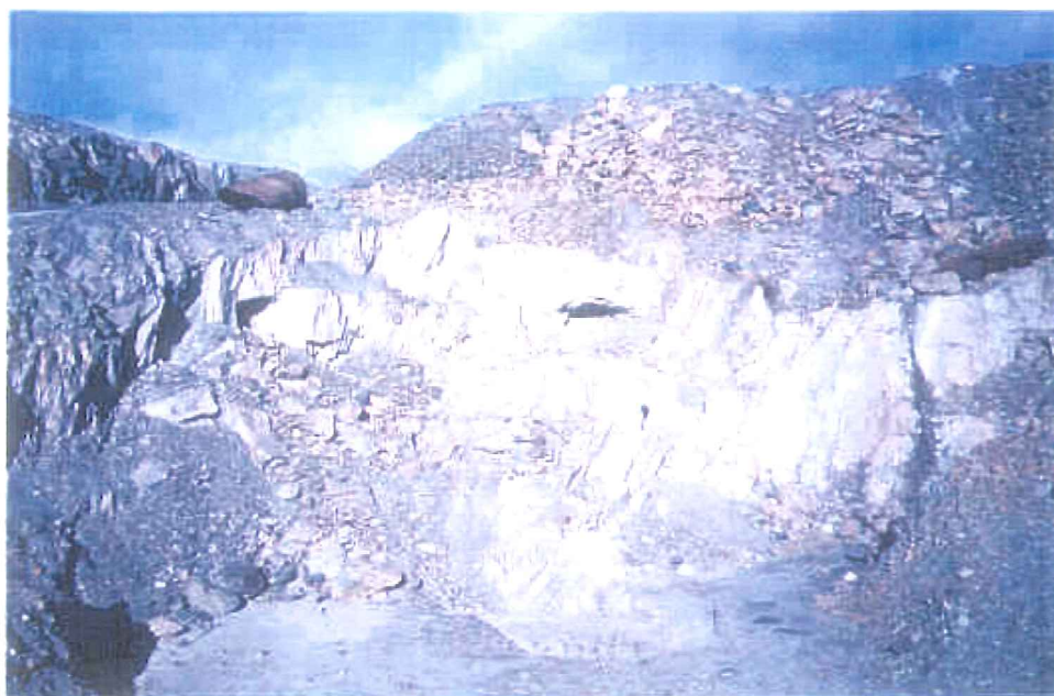
Photo A2-5. B1 Pit looking north-east, showing two underground drifts (2-09) on the northern wall of the pit. Also shows the proximity to bedrock surface.
