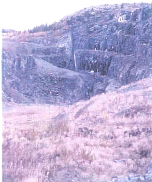
Photo A4-12. AI Pit, looking south-west, showing the benches on the south-western wall.
