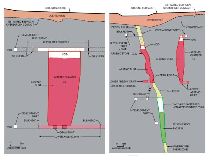
Plate 1-4: Schematic Vertical Sections of Arsenic Stope C212 and Arsenic Chamber 10 Area to Describe Common Underground Terminology (existing conditions)
