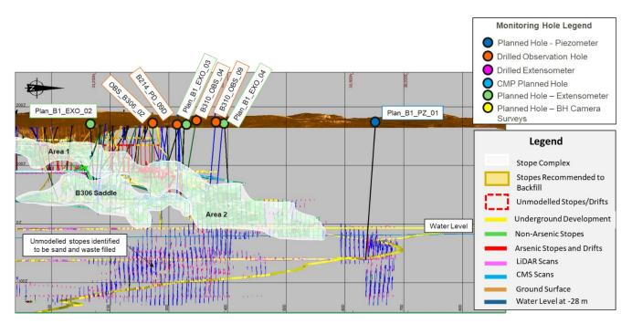
Plate 5-3: Section View (looking west) of Planned Underground Monitoring Locations in B1 Pit Area
