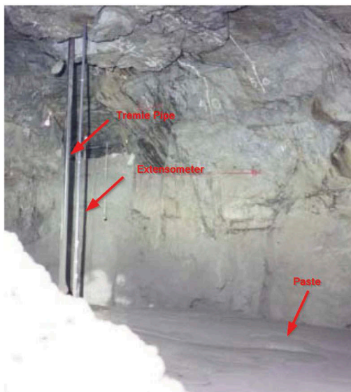
Figure 7. Image of the tremie pipe and extensometer taken with underground camera.
