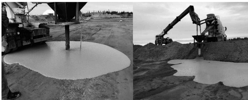
Figure 5. Full scale SCC trial batching on the surface.
