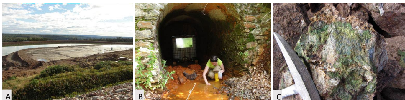
Fig. 4. Three examples of Sb mining sites. A. Tailings at currently operating Beaver Brook antimony mine, Newfoundland, deposited in 2012. The most common Sb host in tailings is stibnite and Sb concentrations in tailings are up to 8 200 mg kg -1 . B. Agnes adit outflow at Poproč Au-Sb deposit in Slovakia. The mine was closed in 1965. Antimony is hosted by Fe (oxyhydr)oxides and is released in water with Sb content up to 380 µg/L in outflow and Sb (>1,200 mg kg -1 in Fe (oxyhydr)oxides. C. Weathered tetrahedrite-rich waste (containing tetrahedrite relics, tripuhyte, roméite) from the historic Ag deposit Špania Dolina Piesky in Slovakia. Photos (A) and (C) taken by Anežka Borčinová Radková and photo (B) by Heather Jamieson.
